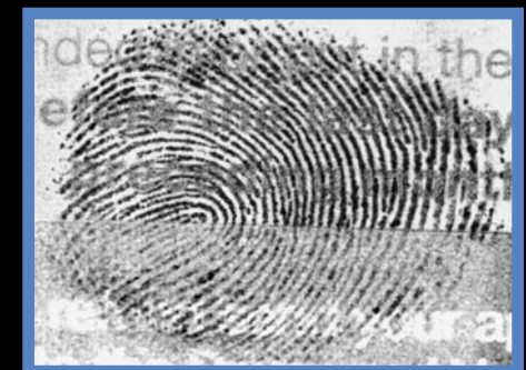
2 Background removal and enhancement using the DCS 4, fingerprint examination system utilising the Crime-lite 8x4 MK2
