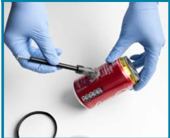
Anti-Stokes powder is applied using a magnetic brush.
